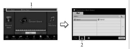
This display can be called up also by pressing the REGIST BANK [+] and [-] buttons simultaneously.
