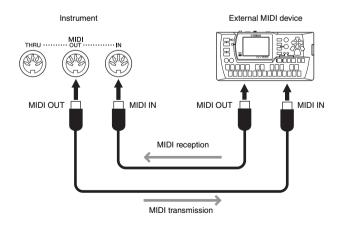
The MIDI settings such as transmit/receive channels on the instrument can be set via [Menu] → [MIDI]. For details, refer to the Reference Manual on the website.
